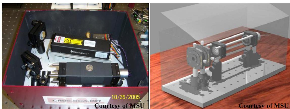
**Figure 5.** A prototype breath acetone analyzer using pulsed-CRDS at 266 nm. *Left:* the instrumental package; *right:* detailed pictorial view of the optical cavity configuration. (Copyright permission [21]).
