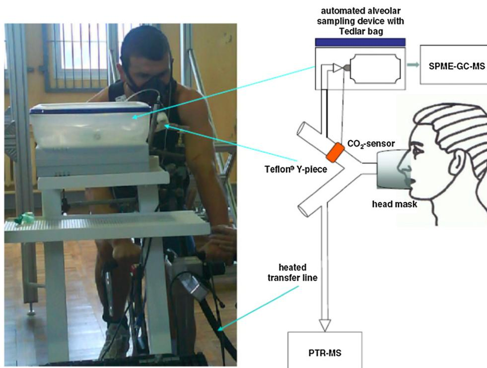
**Figure 2.** Experimental setup and schematic of the breath sampling procedures for real-time breath analysis during exercise using on-line PTR-MS and off-line SPME-GC-MS methods (Copyright permission from Schwoebel *et al* 2011 [73]).
